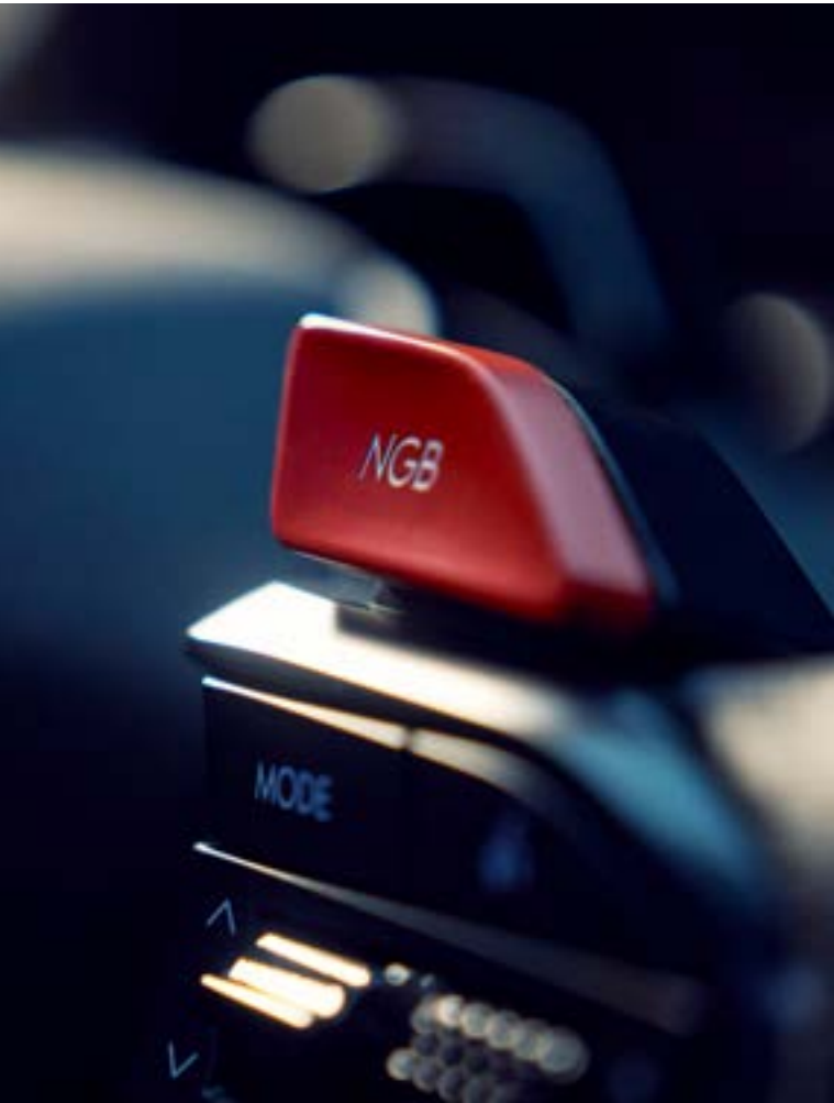
N Grin Boost temporarily increases output by 40 PS.
