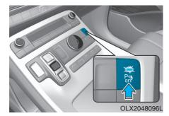
Push the button to turn off the Parking Distance Warning (Reverse) system. The indicator light on the button will turn on.
