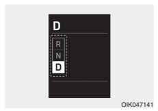
Shift Indicator Pop-up (if equipped) The pop-up that indicates the current gear position is displayed in the cluster for about 2 seconds when shifting into other positions (P/R/N/D).
