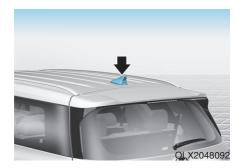
The shark fin antenna receives transmitted data.
