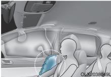
Your vehicle is equipped with a side air bag in each front seat. The purpose of the air bag is to provide the vehicle's driver and the front passenger with additional protection than that offered by the seat belt alone.
