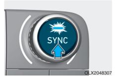
Adjusting the driver and passenger side temperature equally
