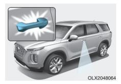
Puddle lamp and door handle lamp With all the doors (and tailgate) closed and locked, the puddle lamp and door handle lamp will come on for about 15 seconds if any of the below is performed.
