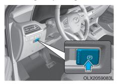
To release the EPB (Electronic Parking Brake), press the EPB switch in the following condition:
