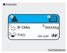
Each symbols and specification on the air conditioning refrigerant label is represented as below:
