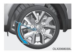
Loosen the wheel lug nuts counterclockwise one turn each, but do not remove any nut until the tire has been raised off the ground.
