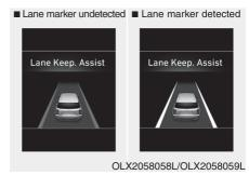
If vehicle speed is over 64 km/h (40 mph) and the system detects lane markers, the color changes from gray to white.
