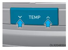
The temperature of delivered air can be set to the desired temperature by pushing the temperature control button.
