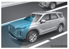
The Lane Following Assist (LFA) system helps detect lane markers on the road with a front view camera at the front windshield, and assists the driver's steering to help keep the vehicle between lanes.
