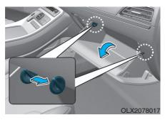
1. With the glove box open, remove the stoppers on both sides.
