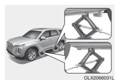
7. Place the jack at the front or rear jacking position closest to the tire you are changing. Place the jack at the designated locations under the frame. The jacking positions are plates welded to the frame with two tabs and a raised dot to index with the jack.
