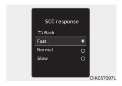
The sensitivity of vehicle speed when following the front vehicle to maintain the set distance can be adjusted. Go to the 'User Settings → Driver assistance → SCC response → Fast/Normal/Slow' on the LCD display. You may select one of the three stages you prefer.
