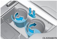
Push the button and the cover opens. Push the buttons and the cup supporter protrudes from the front console. Push in the cup supporter securely after use.
