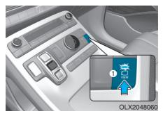
The Surround View Monitor system can assist in parking by allowing the driver to see around the vehicle. Push the button (1, indicator ON) to operate the system. To cancel the system, push the button again (1, indicator OFF).
