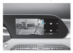
When you touch the icon (1), the top view is displayed on the screen and shows the distance from the vehicle in the back of your vehicle. Touch the icon (1) again, to switch back to the previous screen.
