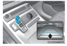
The Rear View Monitor system is a supplemental system that shows the area behind the vehicle on the audio or AVN system screen to assist you when parking or driving.
