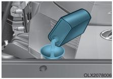
Use only the specified engine oil. (Refer to "Recommended lubricants and capacities" in chapter 8.)
