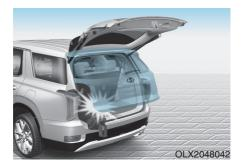
During power opening and closing if the power tailgate is blocked by an object or part of the body, the power tailgate will detect the resistance.
