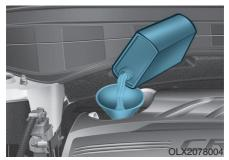
7. If the level is in the D range, add enough engine oil to bring the level up the range.
