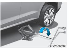
8. Insert the jack handle into the jack and turn it clockwise, raising the vehicle until the tire just clears the ground. This measurement is approximately 30 mm (1.2 in). Before removing the wheel lug nuts, make sure the vehicle is stable and that there is no chance for movement or slippage.
