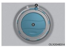
The rear passengers can adjust the direction of air flow from the rear vents on the headlining.
