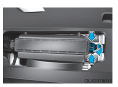
Remove the climate control air filter case while pressing the lock on right side of the cover.
