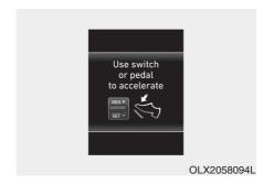
While the Smart Cruise Control (SCC) system is in operation, your vehicle stops behind the vehicle in front when it stops. The message is displayed on the cluster within 3 seconds after the stop and the system will be in the standby position.
