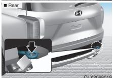
If towing is necessary, we recommend you have it done by an authorized HYUNDAI dealer or a commercial tow truck service. If a towing service is not available in an emergency, your vehicle may be temporarily towed using a cable or chain secured to the emergency towing hook at the front (or rear) of the vehicle.
