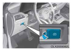
To apply the EPB (Electronic Parking Brake):
