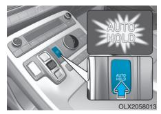
1. With the driver's door, engine hood and tailgate closed, depress the brake pedal and then press the [AUTO HOLD] switch. The white AUTO HOLD indicator will come on and the system will be in the standby position.
