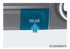
Press the rear climate control button of the front climate control system.
