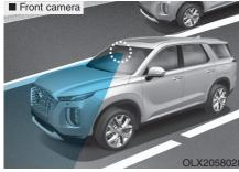
In order for the FCA system to operate properly, always make sure the sensor cover or sensor is clean and free of dirt, snow, and debris.
