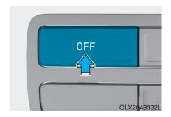
Push the OFF button to turn the rear climate control system off.
