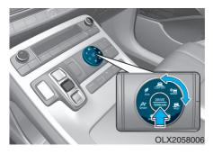
If you press the "DRIVE/TERRAIN" mode button, the driving mode is changed from normal driving control to Multi Terrain Control. You can select SNOW, MUD or SAND mode by rotating the knob. If you press the "DRIVE/TERRAIN" mode button again, the driving mode is changed from Multi Terrain Control to normal driving control.
