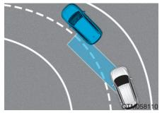
The BCW and BCA systems may not operate properly when driving on a curved road. In certain instances, the system may recognize a vehicle in the same lane.
