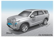
5. Block both the front and rear of the tire diagonally opposite of the tire you are changing.
