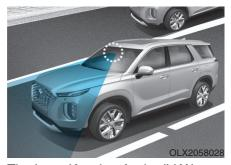
The Lane Keeping Assist (LKA) system with a camera at the front windshield, helps detect lane markers on the road, and assists the driver's steering to help keep the vehicle between lanes.
