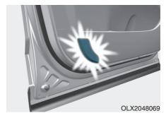
The door courtesy lamp comes on when the door is opened.
