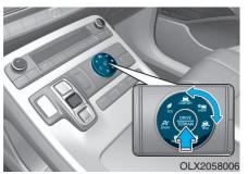
The Four Wheel Drive (4WD) System delivers engine power to all front and rear wheels for maximum traction.
