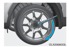
Then position the wrench as shown in the drawing and tighten the wheel nuts. Be sure the socket is seated completely over the nut. Do not stand on the wrench handle or use an extension pipe over the wrench handle.
