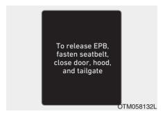
To release EPB, fasten seatbelt, close door, hood and tailgate
