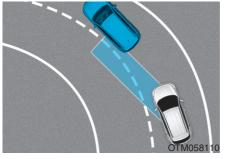
The BCW system may not operate properly when driving on a curved road. In certain instances the system may recognize a vehicle in the same lane.
