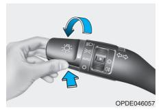
High Beam Assist (HBA) is a system that automatically adjusts the head-lamp range (switches between high beam and low beam) according to the brightness of other vehicles and road conditions.
