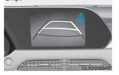
If the vehicle detected by the sensors approaches from the rear left/right side of your vehicle, the warning chime will sound, the warning light on the outside rearview mirror will blink and a message will appear on the LCD display. If the rear view monitor system is in activation, a message will also appear on the audio or AVN screen.
