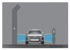
[A] : noise barrier, [B] : guardrail
