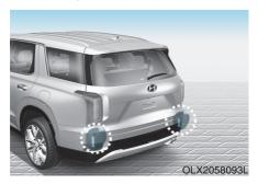
The rear radars are the sensors inside the rear bumper for detecting the side and rear areas. Always keep the rear bumper clean for proper operation of the system.
