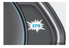
If the EPB malfunction indicator remains on, comes on while driving, or does not come on when the ignition switch is changed to the ON position, this indicates that the EPB may have malfunctioned.
