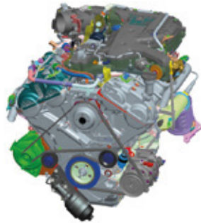
Lambda II 3.8 GDI (ATK) Gasoline Engine
